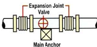
C. At the entrance of a side branch containing an expansion joint into the main line.
