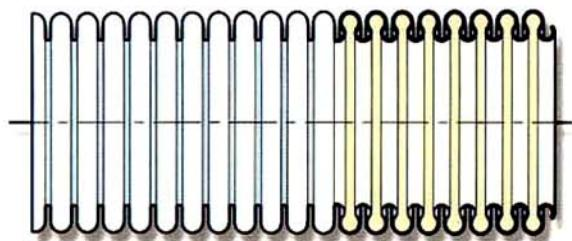
These tubes are excellent in dynamic character and pressure proof. Its flexibility alters the physical image of a metallic tubes.
