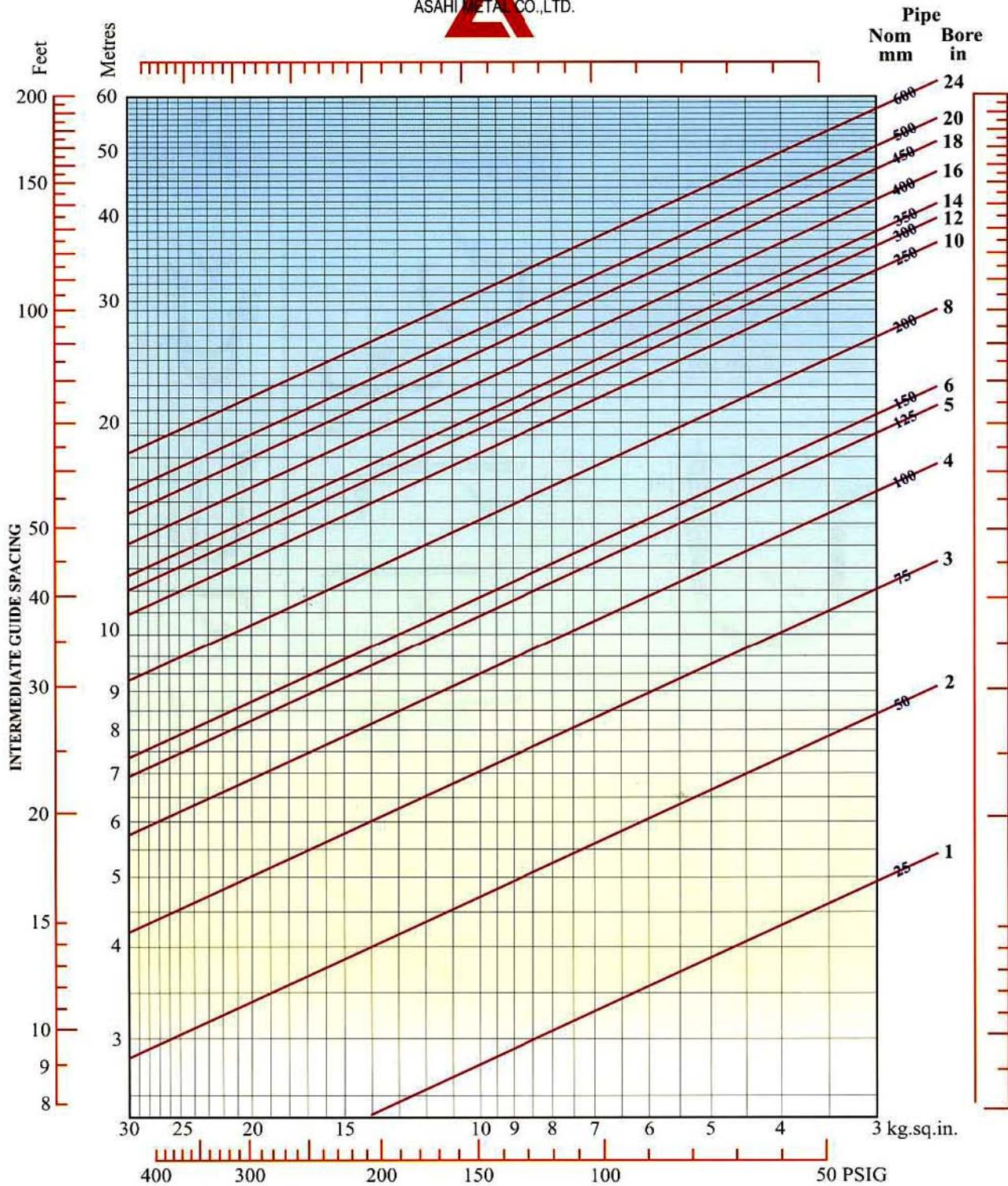
This graph gives the recommended maximum spacing of the intermediate Pipe Guides for application involving AXIAL MOVEMENT Expansion joint line ONLY.
