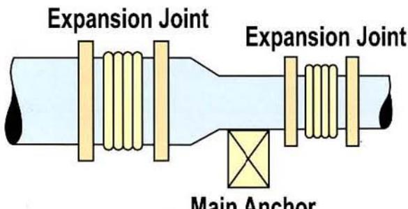
B. Between (2) expansion joints of different sizes installed in the same.
